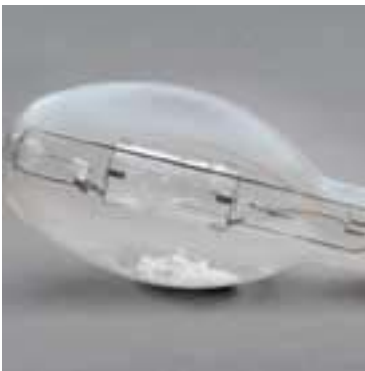
Ruptured arc tube contained within the intact outer jacket of a Venture MP open rated lamp
